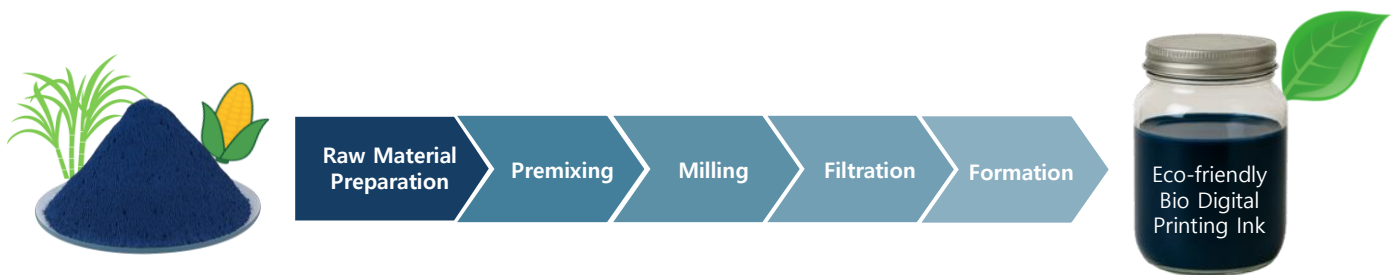
Figure 6-1. Production process for digital printing ink using BioIndigo.
