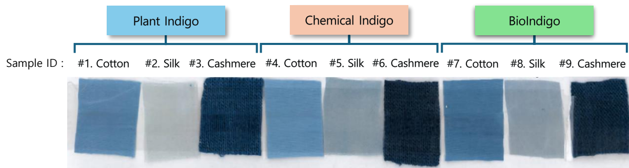
Figure 3-1. Results of the fabric dyeing using different types of indigo dyes.
